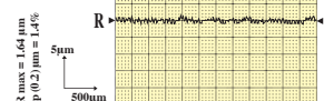
Results of surface finish on 24 pcs. were all within 2.8 microns. (R MAX.)
