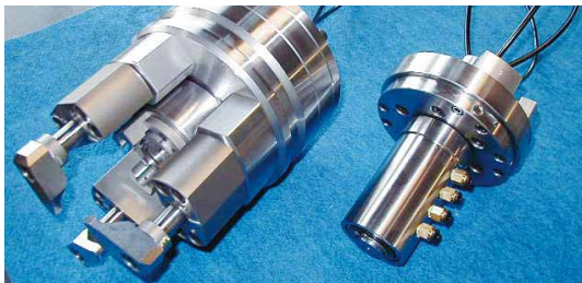
Model Name: HPC-7-01 Kind of Machine: Horizontal Lathe Workpiece: Thin-Ring (Thickness:2mm) Chuck Diameter: 7inch (φ 178mm) Nose: Strait Type Reference: Combination-Chuck, Face Clamping of 3inch+7inch, Built-in Air Cylinder, Max. R.P.M. 2,000, The right side of above is a rotary joint
