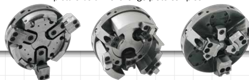
Model Name: AJCA8-12-35-07 Kind of Machine: Combined Machine Workpiece: motor case, die-cast aluminum Chuck Diameter: 12inch (φ 304.8mm) Nose: A2-#8 Reference: work-stopper/rotation direction positioning/ balance weight for exchange plates, Max. R.P.M. 2,500, picture below: exchange plate samples
