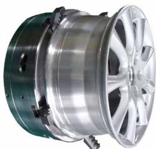
Model Name: K5JA8-20-07 Kind of Machine: Horizontal Lathe Workpiece: Aluminum wheels for automobiles (14inch to 20inch), Remachining (finishing process after coating) Chuck Diameter: 20inch (φ 508mm) Nose: A2-#8 Reference: Cam lever type of 5-jaws, Max. R.P.M. 1,800
