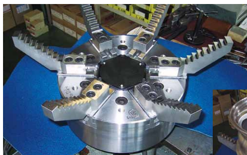
Model Name: Z6JA8-15-120B-03 Kind of Machine: Horizontal Lathe Workpiece: Aluminum wheels for automobiles (14inch to 20inch), Remachining (finishing process after coating) Chuck Diameter: 15inch (φ 381mm) Nose: A2-#8 Reference: Wedge type of 6-jaws
