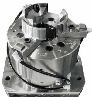
Model Name: STC-8-52 Kind of Machine: Machining Center Workpiece: Gear-Wheel Chuck Diameter: 8inch (φ 203.2mm) Reference: Wedge-type of Stationary Chuck (non-rotation), Trimming inner jaws, Work mounting confirmation structure
