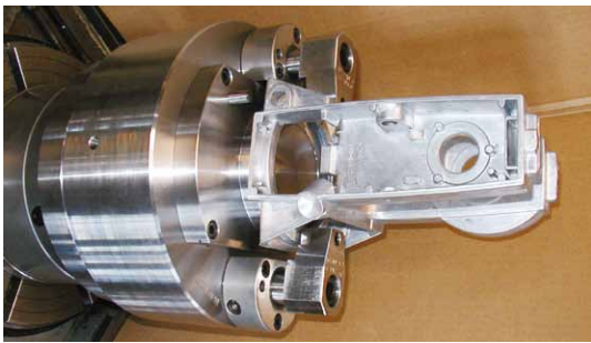
Model Name: HPCJA8-12 Kind of Machine: Combined Lathe (Second Process) Workpiece: Die-Cast Aluminum, Turning & Milling Chuck Diameter: 12inch ( \phi 305\text{mm} ) Nose: A2-#8 Reference: Cam Slot type of 2-jaws (Pull-down, Swivel Face Clamp)
