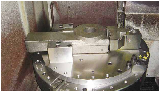
Model Name: HHA11-28-10 Kind of Machine: Vertical Lathe Workpiece: Base Carrier parts for Power Shovel Chuck Diameter: 28inch ( \phi 711\text{mm} ) Nose: A2-#11 Reference: Drives only one in three jaws, Max. R.P.M.400
